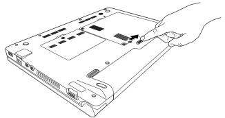
(Sample Illustration) Unlocking the battery release lock
